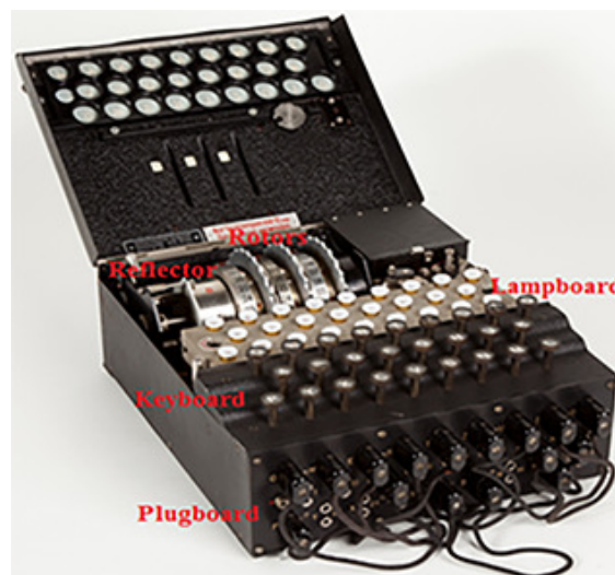
Figure 1: Enigma cipher machine.
